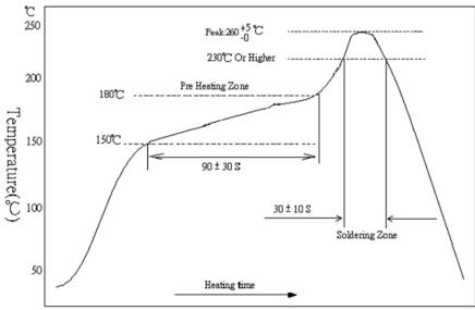
Remark: The peak temperature of soldering heat is 260 +5/-0  $\,\,{}^\circ\!{}_{\rm C}\,$  for 10 seconds
